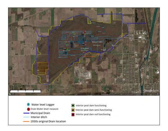
Figure 3. Locations of Water-level loggers managed by 8Tree Inc. and the location of manual water-level measurements within the Beiderman municipal Drain are indicated on the map. Interior Beaver Dams, interior ditches, and the locations of each constructed peat dam and their evaluated conditions as of 2021-2022 are also indicated.
